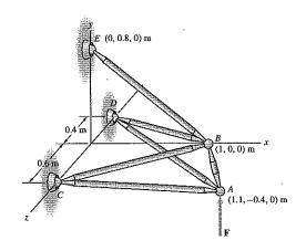
**Solution:** The important points in this problem are A (1.1, -0.4, 0), B (1, 0, 0), C (0, 0, 6), and D (0, 0, -0.4). We do not need point E as all of the needed unknowns converge at A and none involve the location of point E. The unit vectors along AB, AC, and AD are
