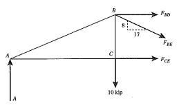
**Problem 6.39** The Howe bridge truss is loaded as shown. Use the method of sections to determine the axial forces in members BD, CD, and CE.
