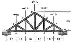
**Solution:** The strategy is to proceed from end A, choosing joints with only one unknown axial force in the x- and/or y-direction, if possible, and if not, establish simultaneous conditions in the unknowns.
