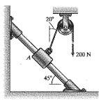
**Solution:** The pulley does not change the tension in the rope that passes over it. There is no friction between the slider and the bar.
