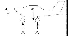
**Problem 18.4** The Boeing 747 begins its takeoff run at time t=0. The normal forces exerted on its tires at A and B are  $N_A=175$  kN and  $N_B=2800$  kN. If you assume that these forces are constant and neglect horizontal forces other than the thrust T, how fast is the airplanes moving at t=4 s? (See Active Example 18.1.)
