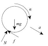
**Problem 18.49** The 5-lb horizontal bar is connected to the 10-lb disk by a smooth pin at A. The system is released from rest in the position shown. What are the angular accelerations of the bar and disk at that instant?
