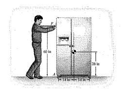
**Solution:** Assume that the refrigerator rolls without tipping. We have the following equations of motion.
