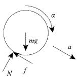
**Problem 18.34** A thin ring and a homogeneous circular disk, each of mass m and radius R, are released from rest on an inclined surface. Determine the ratio  $v_{\rm ring}/v_{\rm disk}$  of the velocities of the their centers when they are rolled a distance D.
