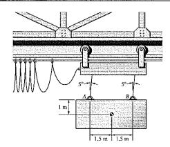
**Solution:** From Newton's second law:  $F_x = 800a$  N. The sum of the forces on the load:
