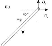
**Problem 18.19** The 5-kg slender bar is released from rest in the horizontal position shown. At the instant when it has rotated 45°, its angular velocity is 4.16 rad/s. At that instant, determine the magnitude of the force exerted on the bar by the pin support. (See Example 18.4.)
