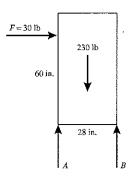
**Problem 18.2** Solve Problem 18.1 if the coefficient of kinetic friction at A and B is  $\mu_k = 0.1$ .
