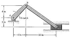
**Solution:** Choose a coordinate system with origin at A and y axis vertical. Let C' denote the instantaneous center. The instantaneous center for bar AB is the point A, by definition, since A is the point of zero velocity. The vector AB is  $\mathbf{r}_{B/A} = 4\mathbf{i} + 4\mathbf{j}$  (in.). The velocity at B is
