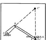
**Problem 17.78** Bar AB rotates at 12 rad/s in the clockwise direction. Use instantaneous centers to determine the angular velocities of bars BC and CD.
