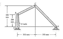
**Solution:** The strategy is analogous to that used in Problem 17.36. The radius vector AB is  $r_{B/A}=200j$  (mm). The angular velocity of AB is  $\omega=-12k$  (rad/s). The velocity of point B is
