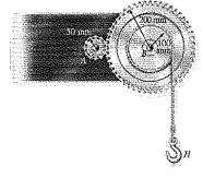
**Problem 17.2** The angle  $\theta$  (in radians) is given as a function of time by  $\theta = 0.2\pi t^2$ . At t=4 s, determine the magnitudes of (a) the velocity of point A and (b) the tangential and normal components of acceleration of point A.
