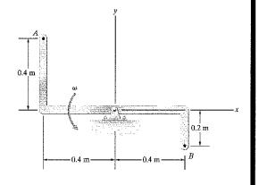
**Problem 17.21** The bracket is rotating about point O with counterclockwise angular velocity  $\omega$ . The magnitude of the velocity of point A relative to point B is 4 m/s. Determine  $\omega$ .
