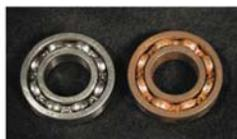
**Treated with CorrosionX (left) and untreated. Exposed to saltwater spray for two weeks**
